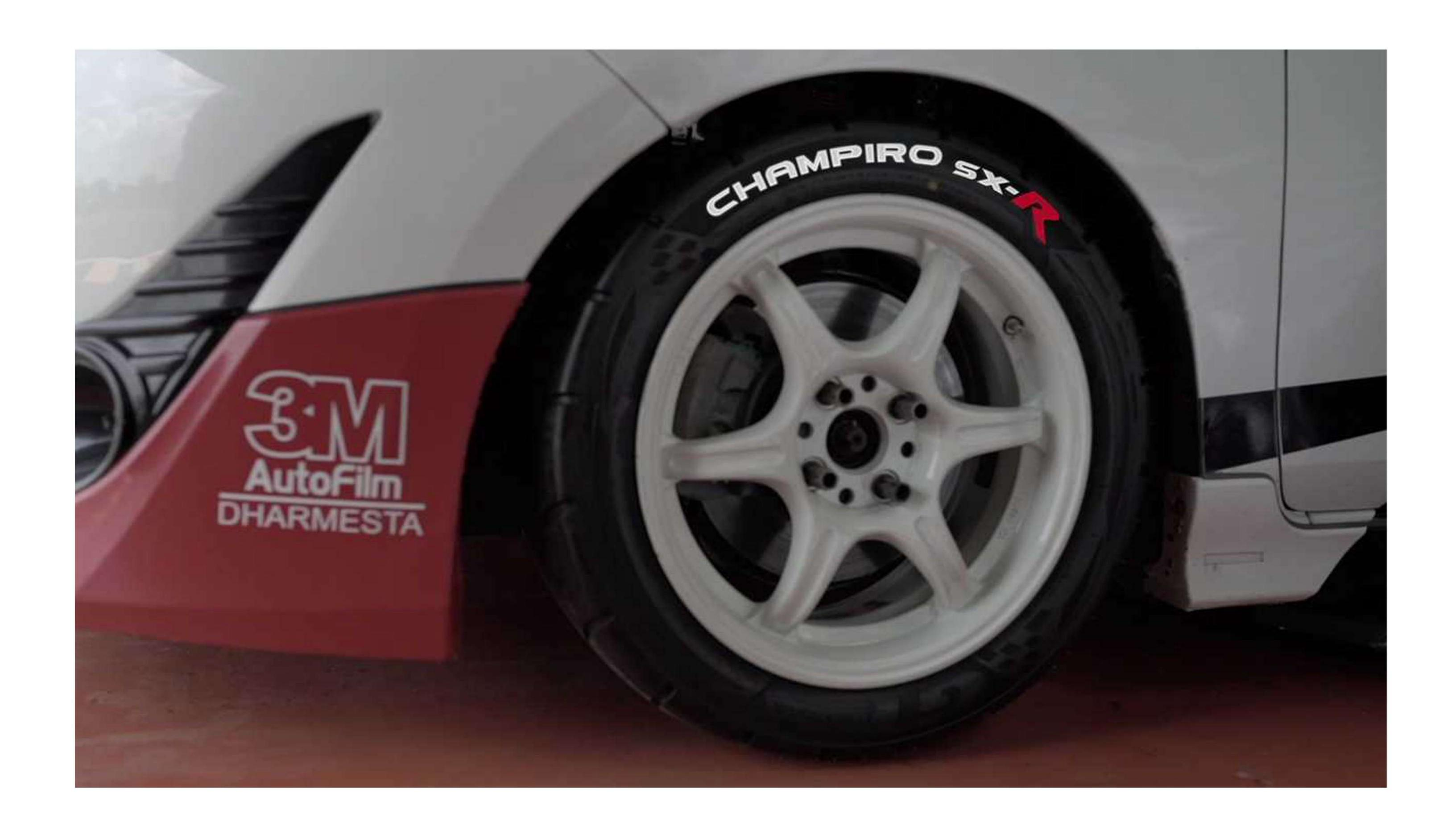
Another innovation for the GT Radial Champiro SX-R is the Special Tread Formula technology which has been tested and proven to improve stability and very competitive performance and adopts High-module Polyester Carcass technology to avoid deformation at high temperatures. The wavy pattern groove design provides precise cornering performance.
